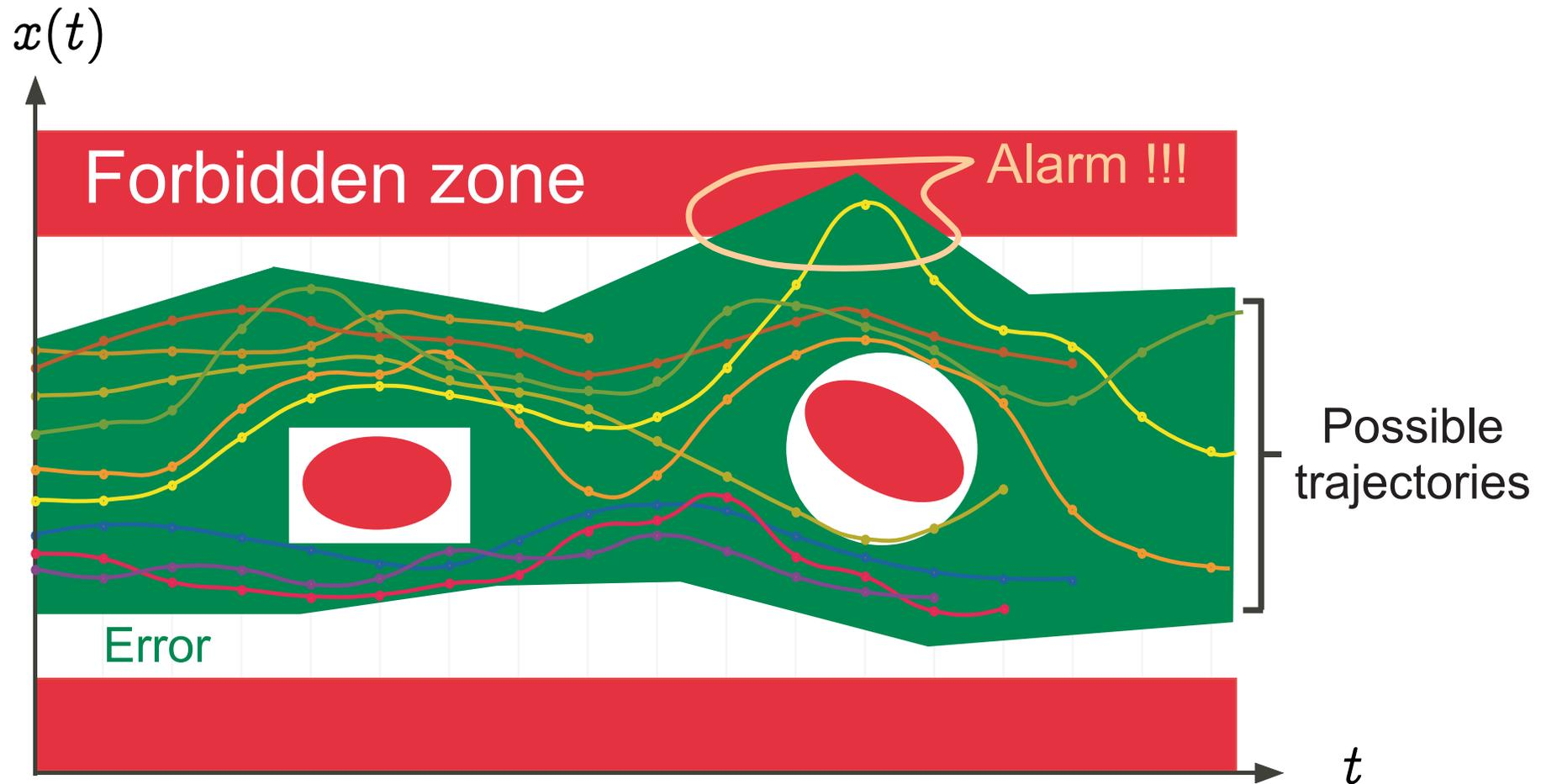
An alarm can originate from an over-approximation
