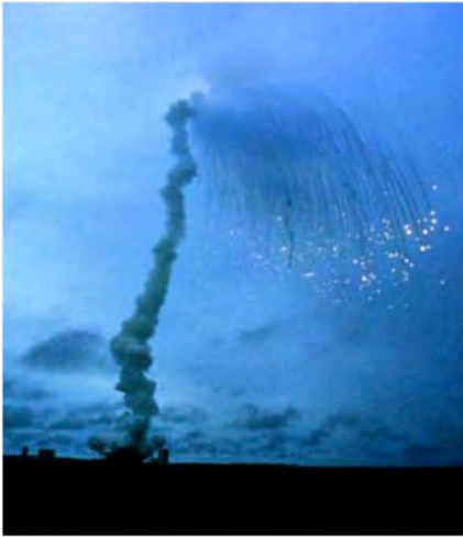
Ariane 5.01 failure (overflow error)
