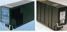
An Air Data Inertial Reference Unit (ADIRU) is a key component of the integrated Air Data Inertial Reference System (ADIRS), that supplies air data (airspeed, angle of attack and altitude) and inertial reference (position and attitude) information to the pilots' Electronic Flight Instrument System displays as well as other systems on the aircraft such as the engines, autopilot, flight control and landing gear systems
